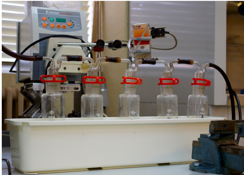
Figure 2.5 Train of bubbling flasks in ice bath. In the background: peristaltic pump.
