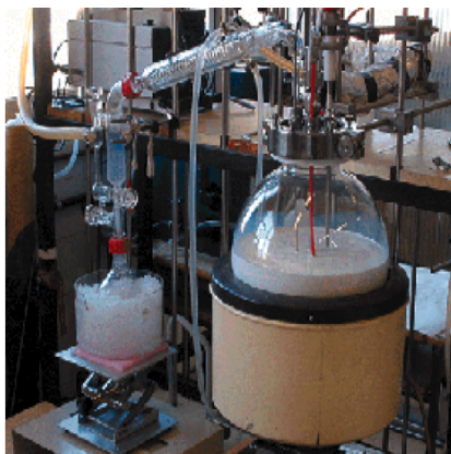
Figure 2.1: An emulsifier where Controlled Radical Polymerization can take place.
