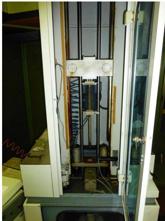
Figure 2.31: The Fractovis 6789, the machine used to impact the samples.
