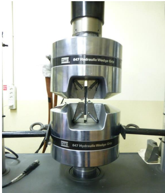
Figure 2.14: the machine used for the compression tests.
