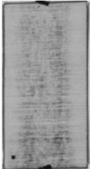
Figure 2.9: Results of ultrasonic scan over NOP_DB1 plate
