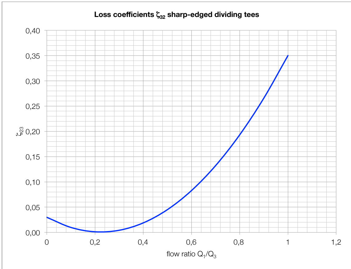
Graph 7: Loss coefficients \zeta_{32} sharp-edged dividing tees
