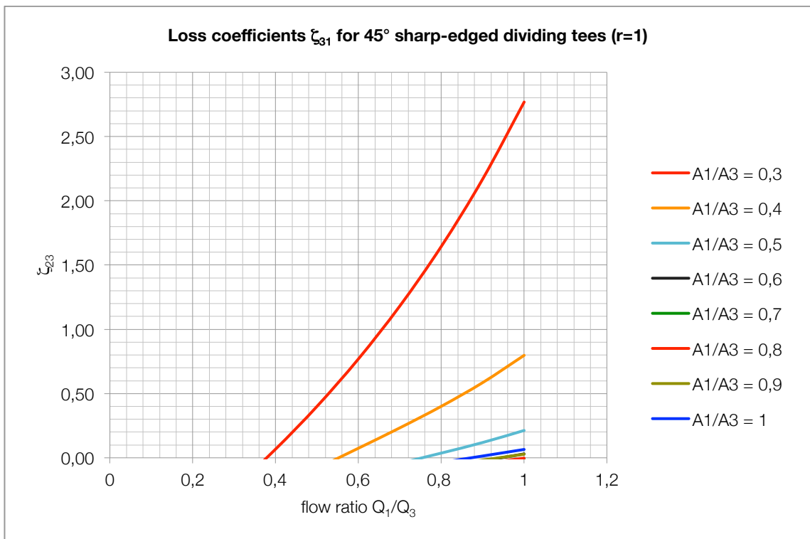
Graph 11: Loss coefficients \zeta_{31} for 45 degrees sharp-edged dividing tees ( r=1 )
