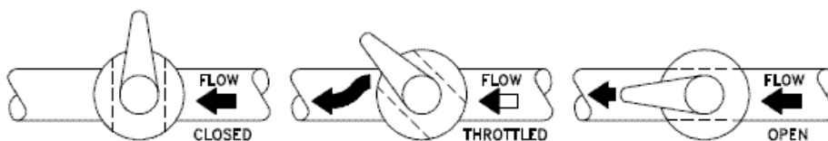
Figure 26: Throttling positions of plug valves
