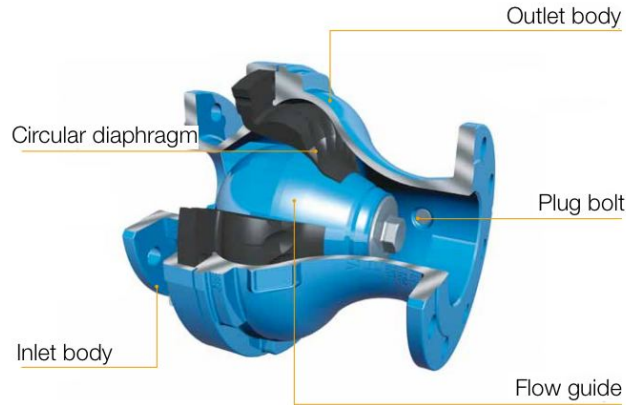
Figure 55: schematic view of VAG TOP-STOP valve
