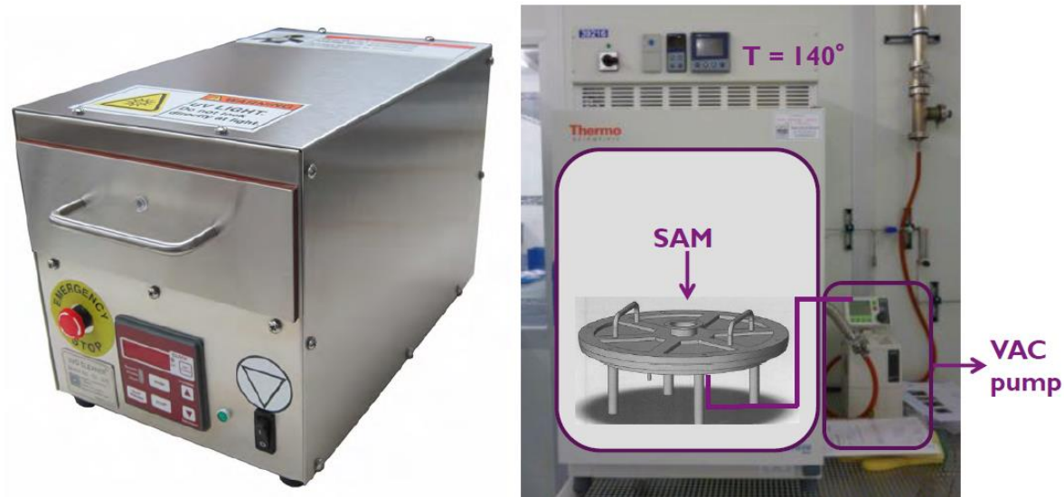
Figure 3.1 - The UvO cleaner (left) and the Silanization Oven (right) used during the research 96 .
