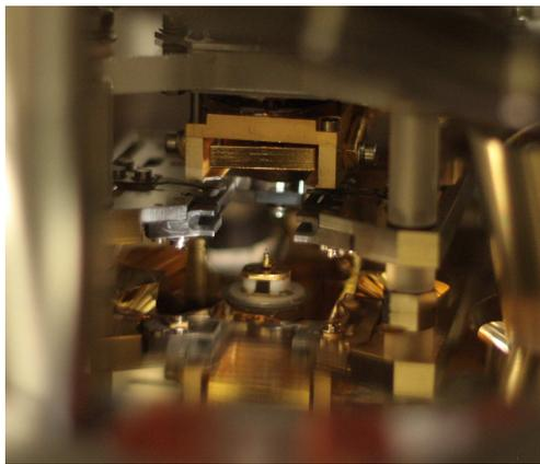
**Figure A.2:** STM sample stage. The tip is placed on top of a cylindrical piezoelectric that allows the scanning of the sample.
