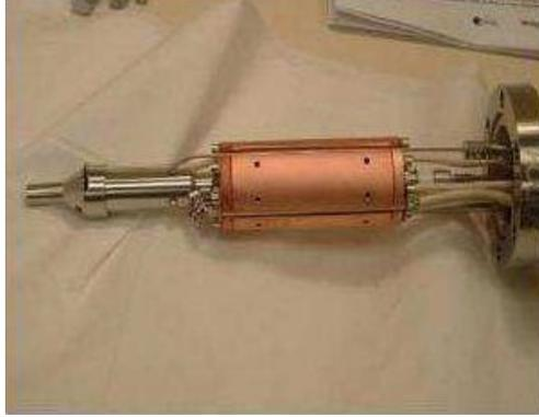
**Figure A.7:** Thermal evaporator, model EFM EVC300. It is visible the copper shroud surrounding the evaporant and the filament.
