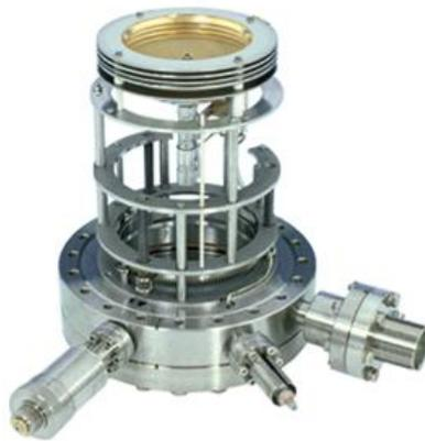
**Figure A.9:** Inner view of the LEED apparatus.
