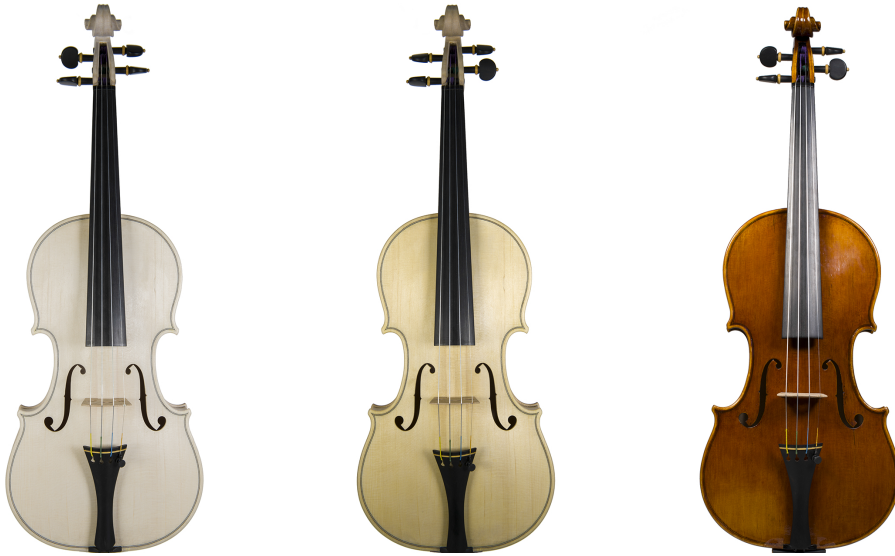
Figure 4.2. The violin in the three steps of the making process. In the white Fig. 4.2(a), with ground coat in Fig. 4.2(b) and varnished in Fig. 4.2(c).
