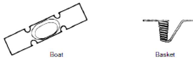
Figure 2.2. Crucible used: the shape on the left is used for Cr evaporation, a molibdenum foil was deformed to obtained it; the basket shape is a tungsten filament, used for gold [42].
