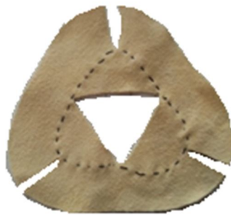
Figure 3.8: deer shaped leaflet. The three cuts on the outer tissue are useful for folding the tissue on the stent
