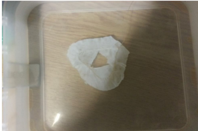
Figure 3.12: shaped tissue with white thread describing the leaflet shape.
