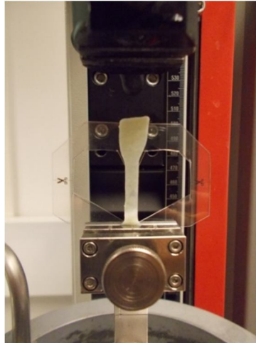
Figure 44: Pericardial specimen during tensile test
