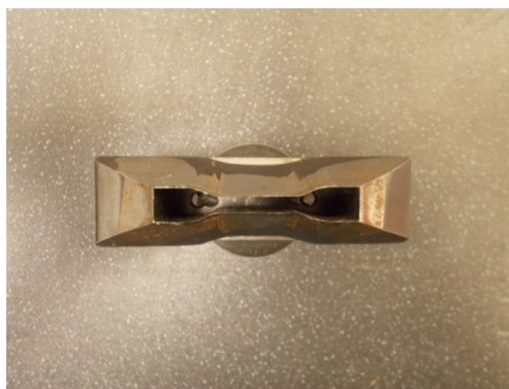
Figure 3.26: Mold used for the realization of the specimens
