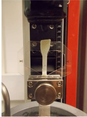
Figure 3.31: Pericardium specimen placed in the machine
