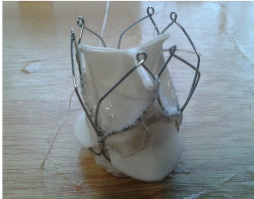
Figure 3.15: leaflets stitched to the stent
