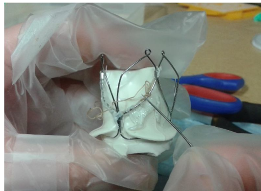
Figure 40: suturing of the tissue to the stent
