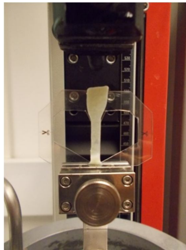
Figure 3.4: Pericardial specimen during tensile test
