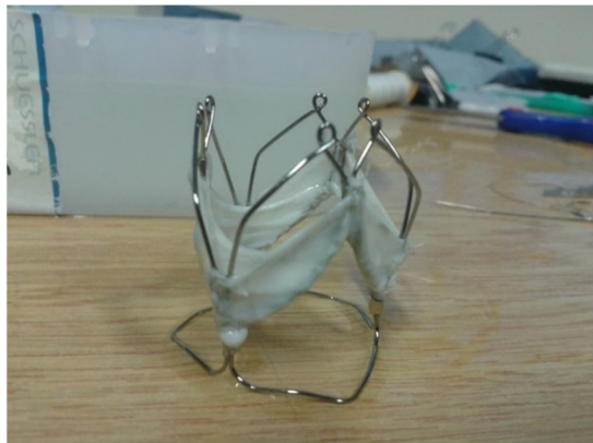
Figure 43: Valve with leaflets made of decellularized pericardium
