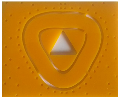
Figure 37: Plastic model realized with laser cutting
