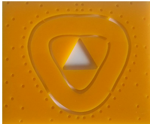
Figure 3.9: Plastic support obtained by laser cutting; all the holes and cuts apart of their function allow water to wet the tissue when dipped into water
