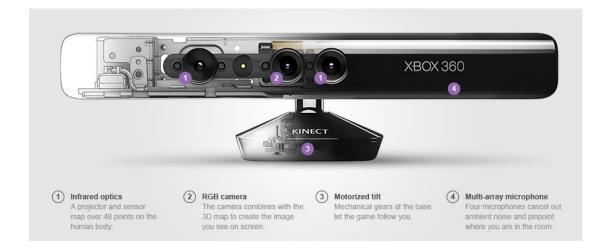
The depth sensor consists of an infrared laser projector combined with a monochrome CMOS sensor, which captures video data in 3D under any ambient light conditions. The sensing range of the depth sensor is adjustable, and the Kinect software is capable of automatically calibrating the sensor based on game play and the player's physical environment, accommodating for the presence of furniture or other obstacles.
