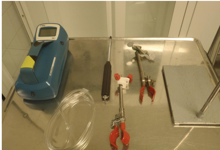
Figure 3.9. Clean instruments. In order from left: P-trak, Tygon piping, telescopic probe, telescopic instrument holder , probe holder.
