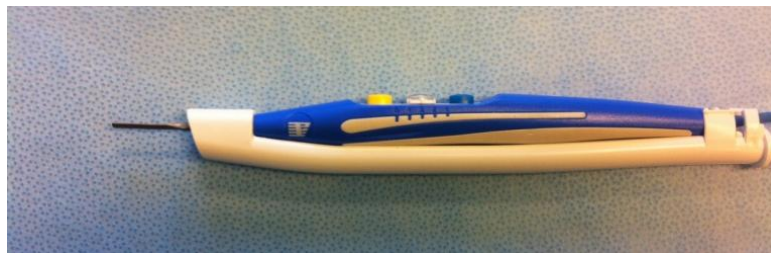
Figure 2.11. Monopolar diathermy attached to local exhaust system
