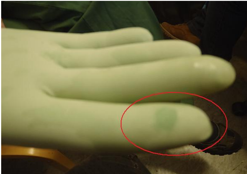
Figure 2.10. The red circle points out a stronger color contrast which is the hole indicator.
