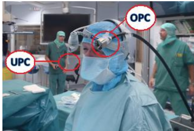
Figure 5.8. The disposition of the two measuring probes near the surgeon's nose in position 3. UPC sampling probe on the left and the isokinetic probe of the OPC on the right.
