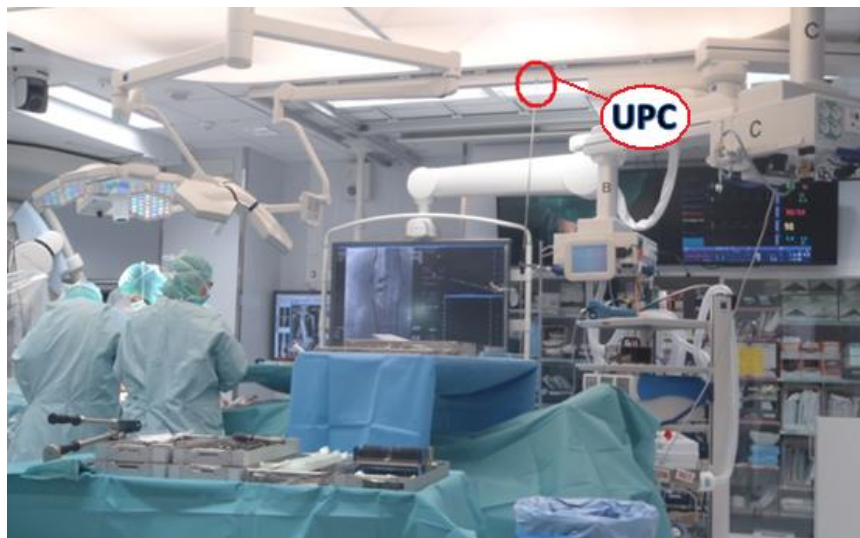
Figure 3.15. UPC (P-TRAK™) positioned in the clean area with the red circle that indicates the position of the telescopic probe placed at the height of 2.80 m, which means at a distance of 20 cm under the H14 HEPA filters.
