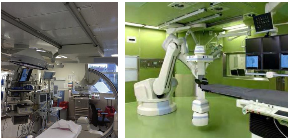
Figure 2.3. On the left, a ceiling mounted C-arm (Schaadt and Landau, (2013)), on the right a floor mounted X-ray scanner (Nollert et al, (2012)).
