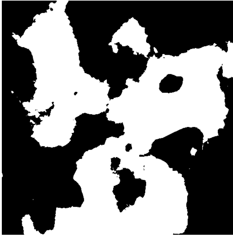
Figure 5.8: Example of map created with Automatic Terrain Generation. The parts in black are obstacles, meanwhile the white places compose the free space.
