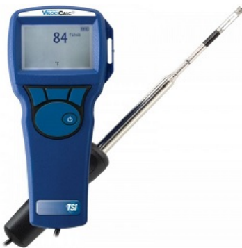
Figure 5.13: Multi-purpose instrument for measuring the speed with hot-wire anemometer and its technical specification (Source TSI Inc.)
