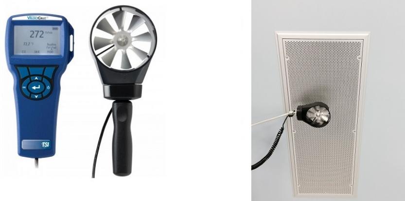
Figure 5.15: Vane anemometer and its utilization during the test
