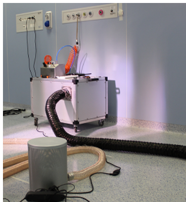
Figure 5.9: Fan and aerosol generator used in during the experimental campaign
