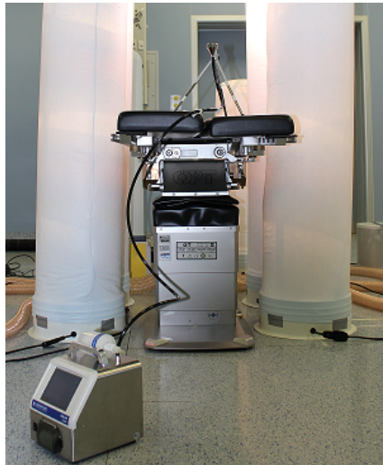
Figure 5.12: The OPC Solair 3100+ (on the floor) and the isokinetic particle sampling probe with its tripod (on the table) used during experimental tests
