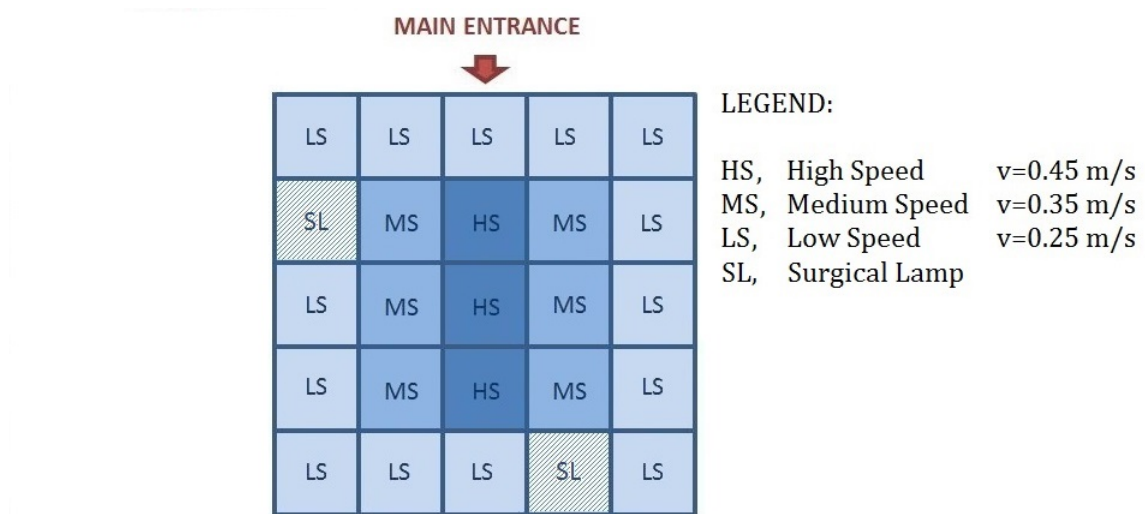
Figure 4.18: Filters of the ceiling diffuser system, different type with different air supply velocities for the scenarios A1 and A2
