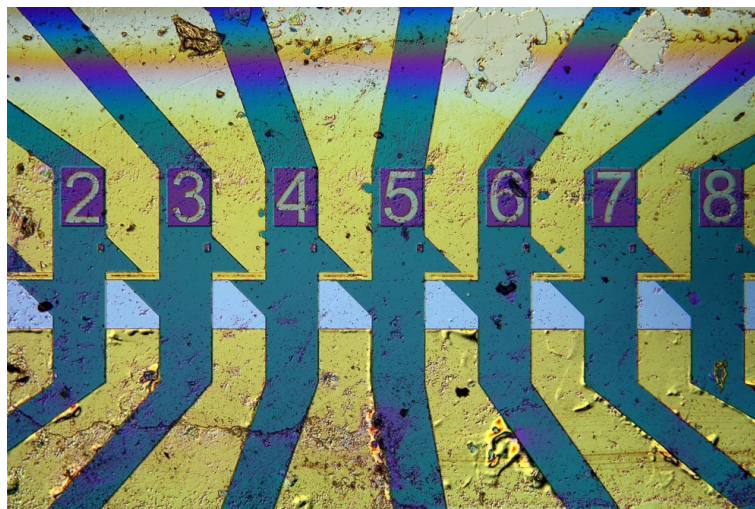
Figure 5.11: Magnetic Tunnel Junctions, array of devices on single die, photograph by optical microscope
