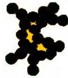
figure 1.13: schematic example of occluded rubber for a carbon black aggregate with high structure
