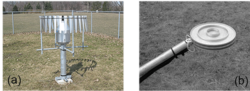
Figure 3.1: Snow gauge of the Waterloo University, Ontario, Canada (a) and a hotplate snow gauge (b)
