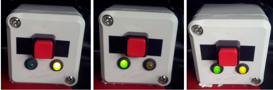
Figure 3.5: The three LED configurations associated to the driving modes. From left to right: driven by user, driven by PC, driving disabled
