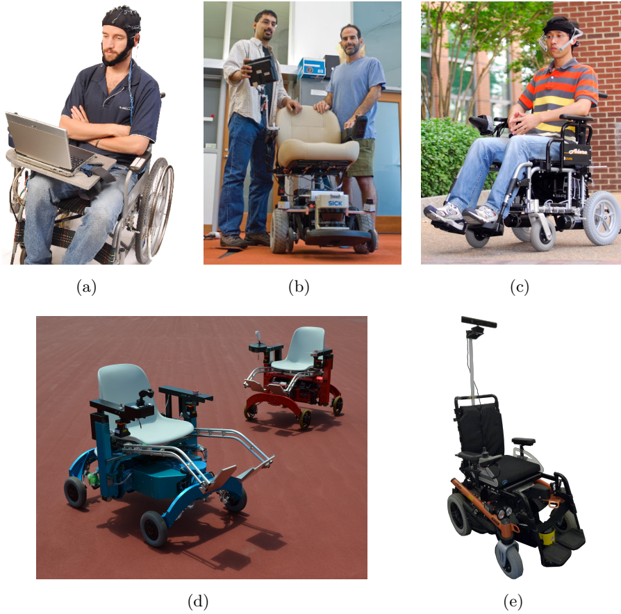
Figure 2.3: Some recent examples of robotic wheelchair: BCW (a), MIT Wheelchair (b), TDS-PWC (c), RT-Mover (d) and Intelligent Wheelchair (e)
