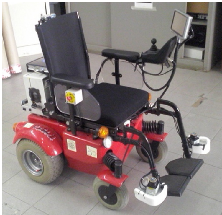
Figure 3.9: The complete LURCH robotic system
