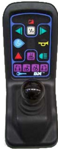
Figure 3.4: A DX-REM34: command panel
