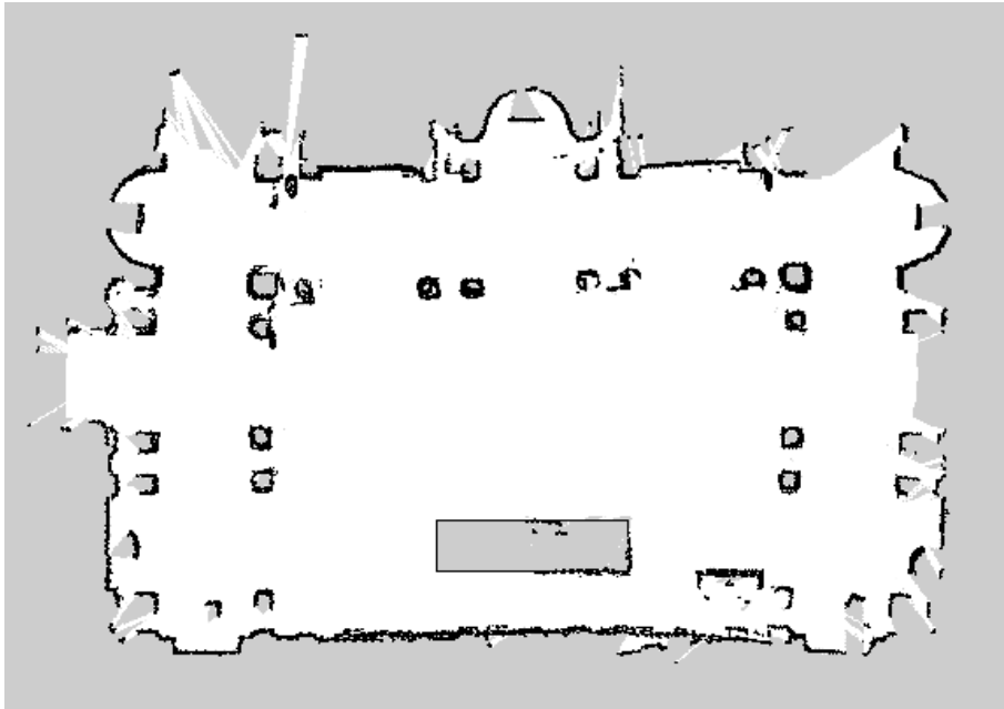
Figure 4.12: An example of map generated by gmapping for LURCH
