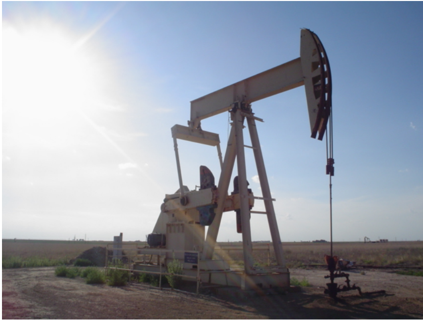
Figure 1.1: A pumpjack in Texas: a pumpjack is an onshore overground drive for a piston pump in an oil well.
