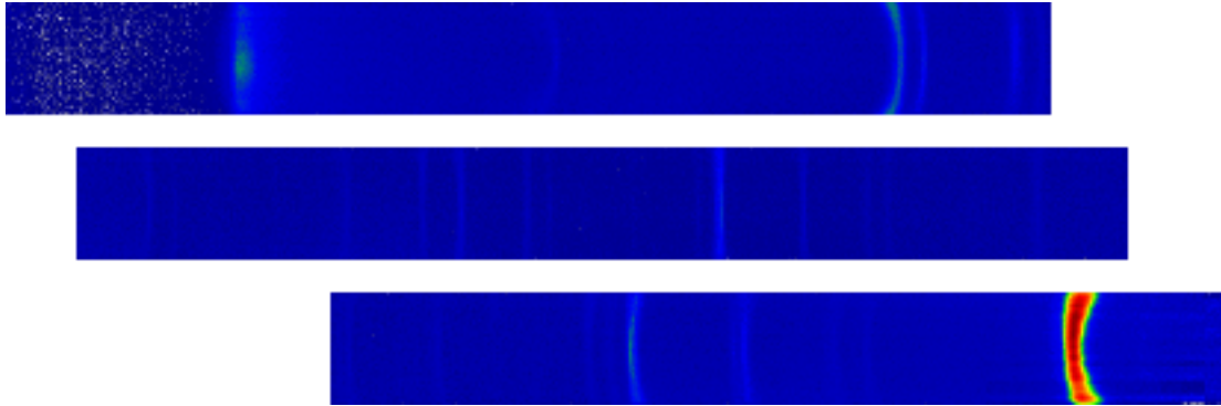
Figure 4.4: Image of a single scan collected on \text{EuTiO}_3 sample at D2B beamline at ILL. The scan has been cut into three slices for printing need.
