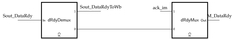
Figure 4.7: Wrapper logic for the DataRdy signal
