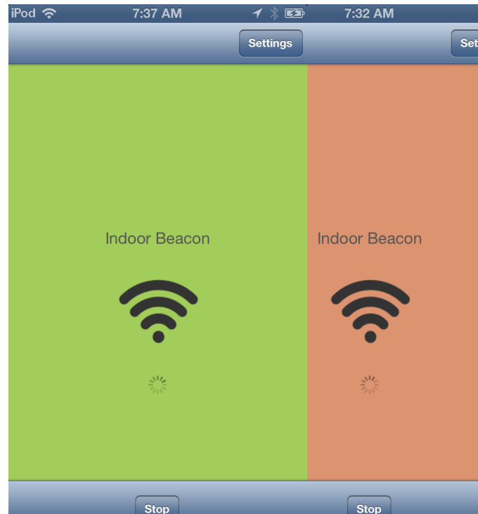
Figure 4.1: Beacon App changing state from central (green) to advertising (orange) one.
