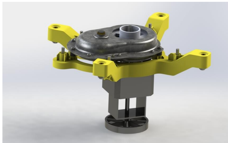
Figure 0-19: Motor support as a structural part
