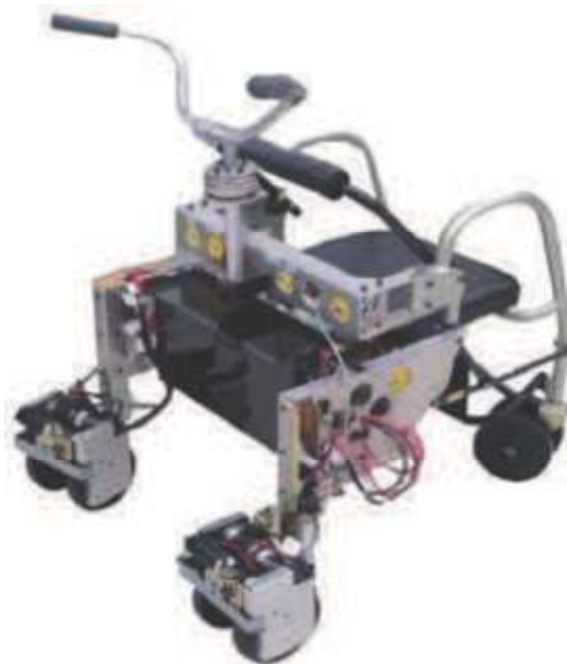
FIGURE 3.10: The hybrid walker. The User can push the walker or sit on it as if it was a wheelchair.
