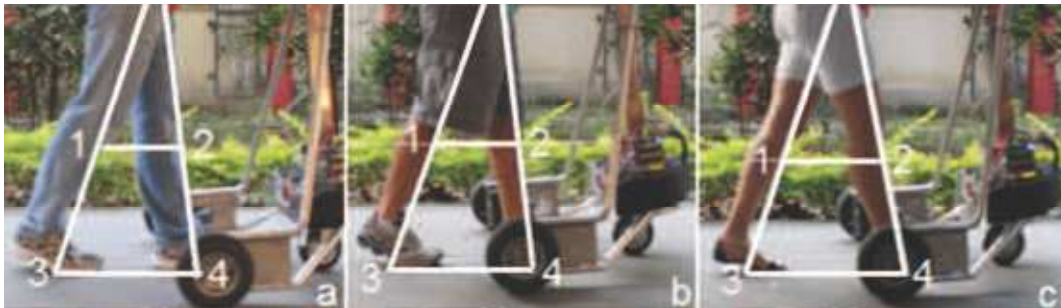
FIGURE 4.14: 3 Users while performing the test, on the picture are marked the four point that allow to calculate the corrective coefficient CC. Respectively are representing: (a) a tall person, (b) an average height person (c) a short person.
