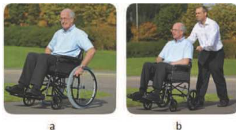
FIGURE 3.9: Pictures representing the possible configuration of wheelchair propulsion: User propelled in (a) and attendant propelled in (b)
