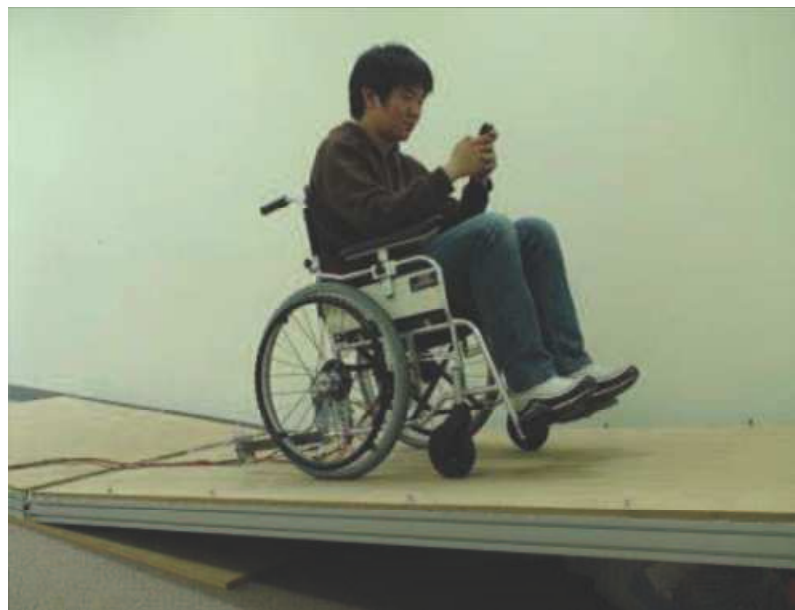
FIGURE 3.4: The CGPAW wheelchair while testing the control on slope. The User is able to check his mobile phone while the wheelchair by itself remains still on slope.
