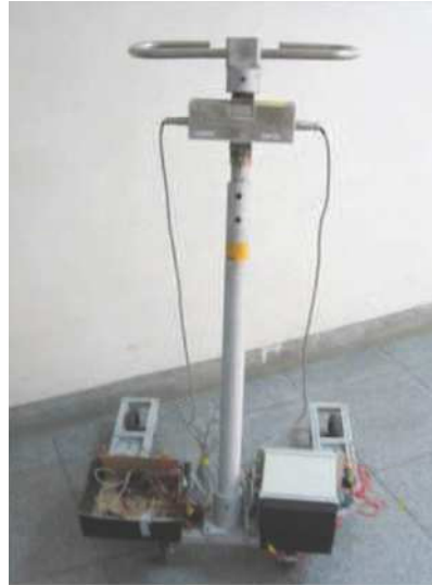
FIGURE 3.12: Picture of the active type SmartWalker developed by KO et al.
