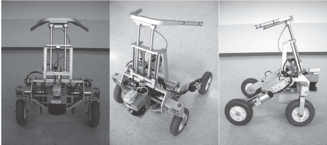
FIGURE 3.13: Pictures of the outdoor intelligent Walking Assistant Robot (WAR)
