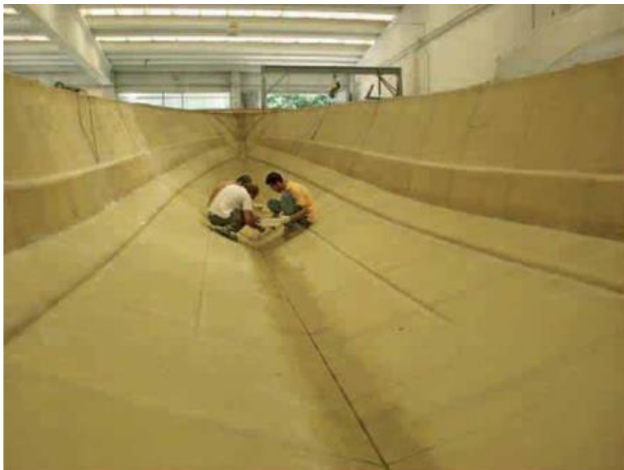
Figure 18: With the use of advanced composites have been able to achieve the shell of large dimensions, greatly reducing the weight and increasing the stiffness
