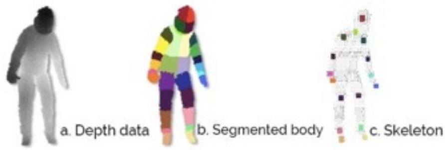
Fig. 11 Representation of the three steps around the Skeleton detection: starting from the 3D points of the body (a), the algorithm segments the body (b) and finally with a weighted average it obtains the Skeleton (c).
