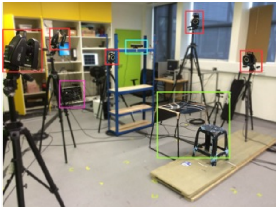
Fig. 26 Laboratory furnished with: red square the VICON cameras, green square the table, light blue square the Kinect, purple square the processing stack.
