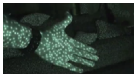
Fig. 9 IR speckles recorded with an IR camera.
