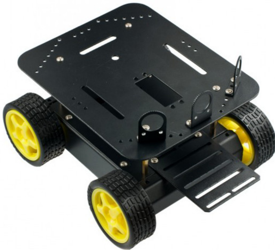
Figure 4.6.: The Pirate robot chassis, without any component mounted with the exception of motors and wheels.
