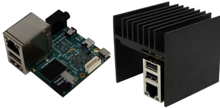
Figure 4.5.: An ODROID-U2 board without (on the left) and with (on the right) its heatsink case.
