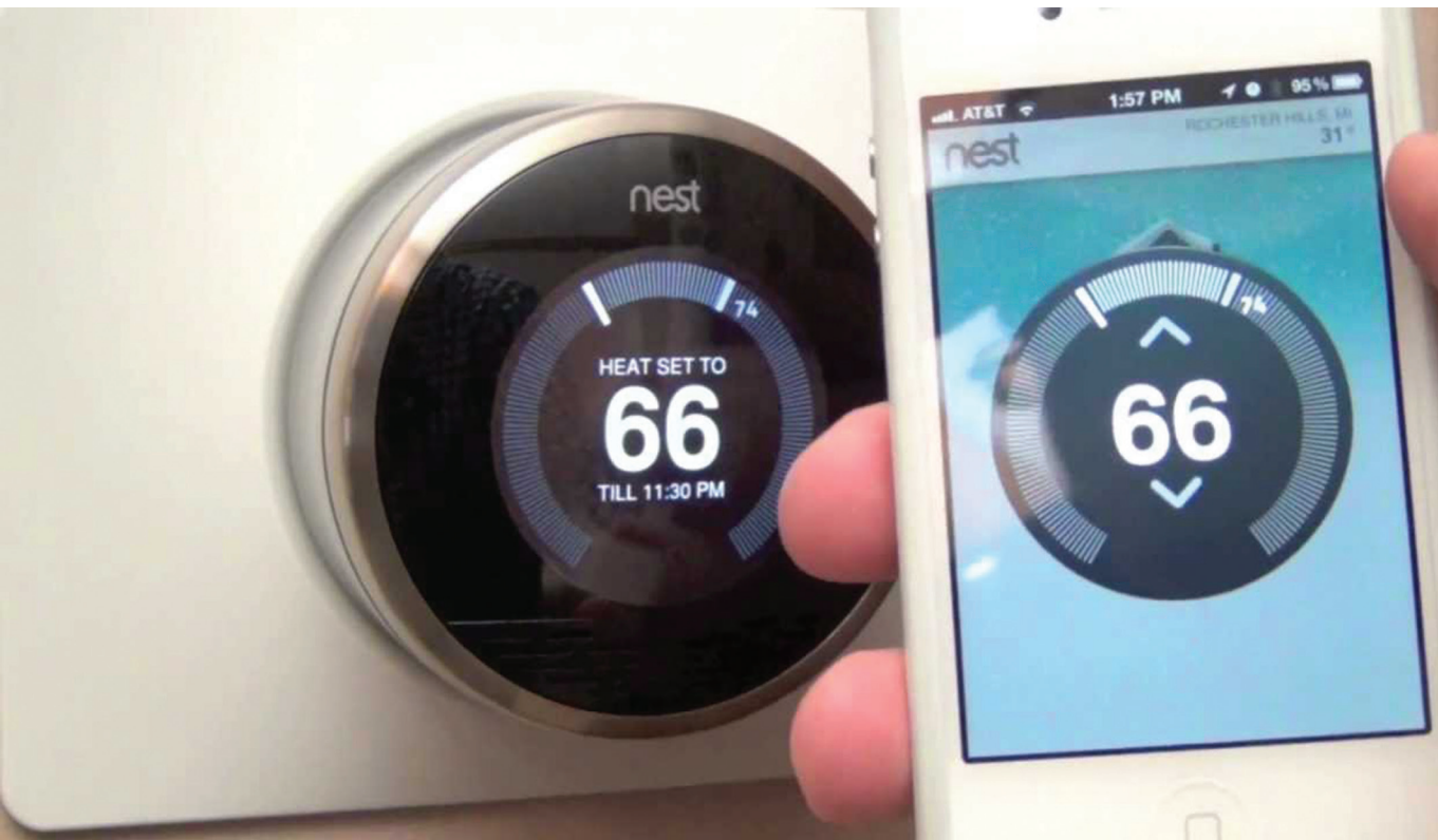
Figure 23. Nest Learning Thermostat, the connected thermostat that schedules itself and can be controlled by an app.
