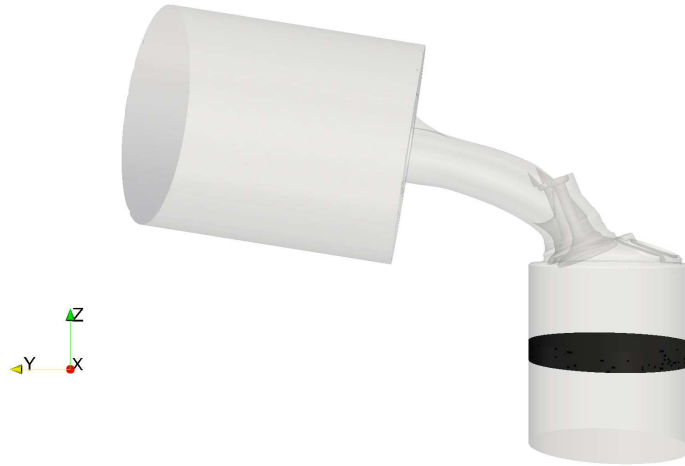
Figure 4.3: Porous media within the cylinder
