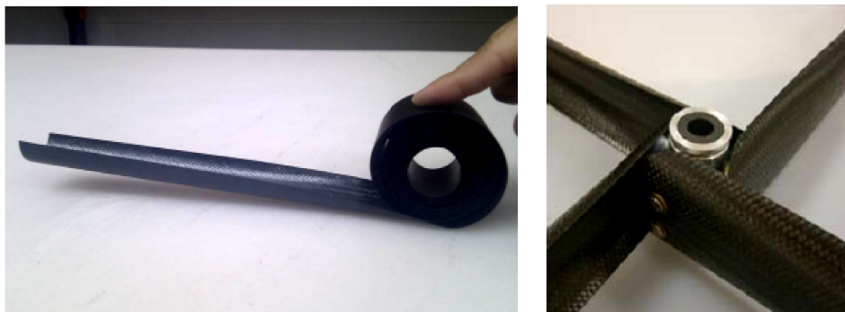
Figure 2.2: Open-section CFRP bistable boom [13] and co-attachment to spindle [14]
