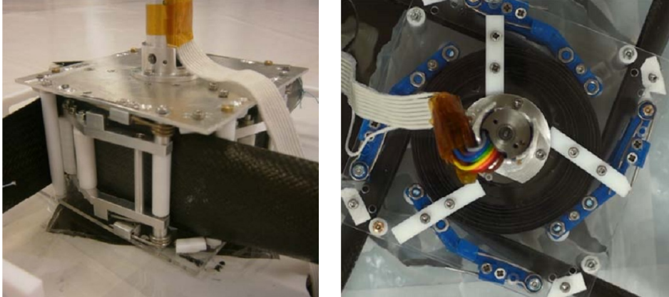
Figure 2.3: The CFRP boom deployment mechanism (left) and a detail of the coiled booms [14]
