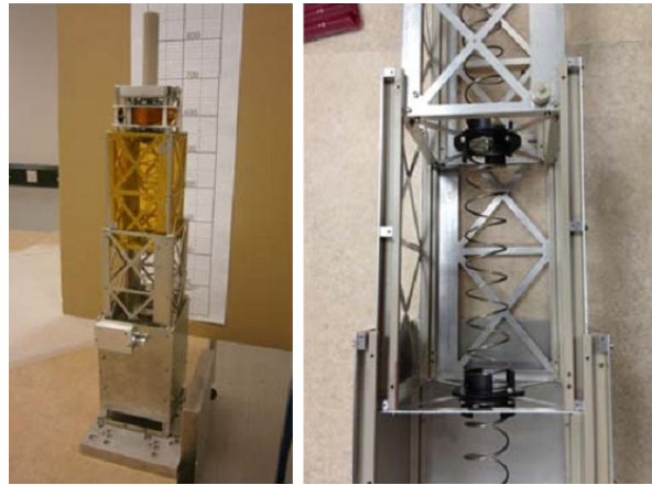
Figure 2.4: The telescopic deployment system designed by SSC and a detail of the compression springs used as actuators [14]
