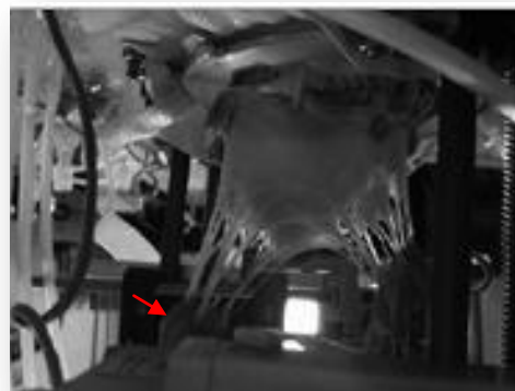
Figure.2: A) Schematic of the test bench P): hydraulic piston pump; V-A: are respectively the ventricular chamber and atrial chamber; I: system that simulates the resistance of the systemic circulation; A: preload. B) Mitral valve housed in a support system and anchored to papillary muscles of the gripping systems (red arrow).
