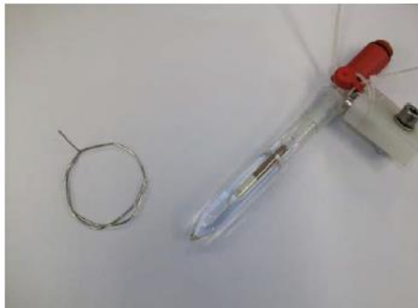
Figure 3.4 – Silver/silver chloride RE and platinum coil CE
