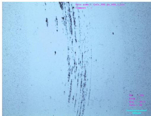
Figure 4.18 - Wear track of a CoCrMO sample after a tribocorrosion experiment at applied potential of 0V and under a 3N load with a PE ball as counterpart
