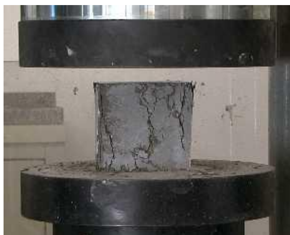
Figure 3.4. Example of compression test on a standard cubic concrete specimen.
