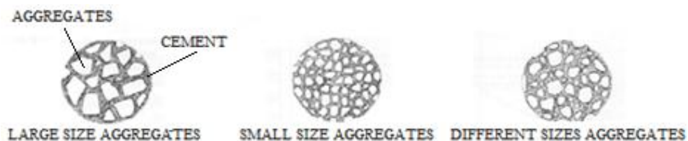
Figure 3.2. Concrete different compositions according to the aggregates size.
