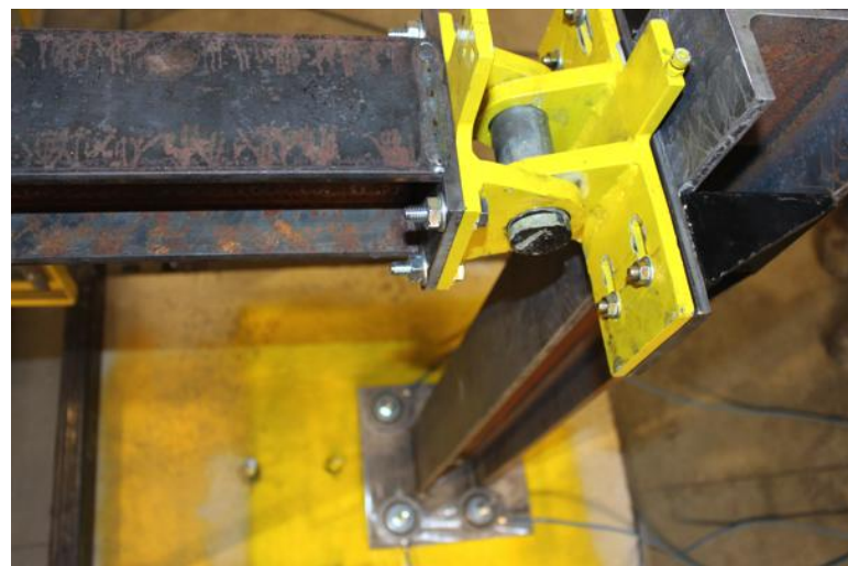
Figure 5.12. Post HEA120 and pushing system.
