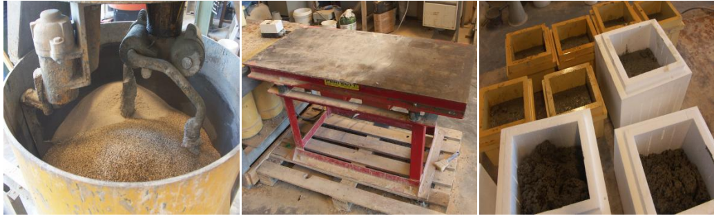
Figure 4.1. Three steps of the concrete production: the mixing machine (on the left), the vibrating table (in the middle) and the molds filled with the mixture (on the right).
