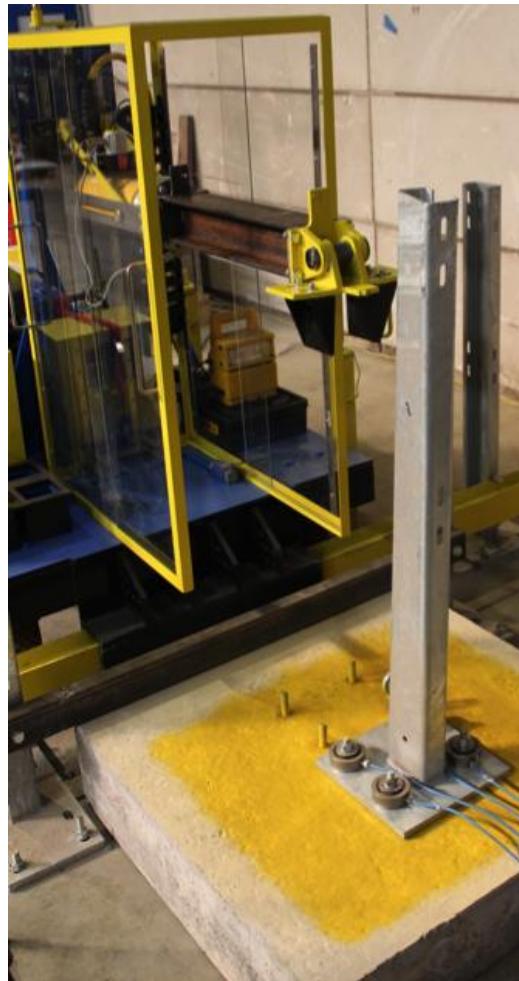
Figure 5.4. Post C125 and pushing system.
