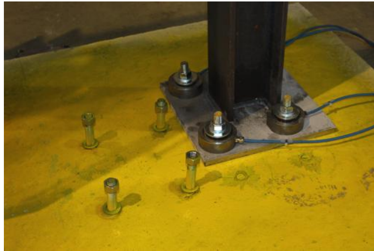
Figure 5.11. Force transducers placed on the anchor bolts of the post HEA120.
