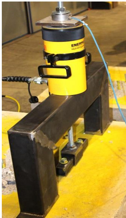
Figure 5.18. Traction test on two anchor bolts.
