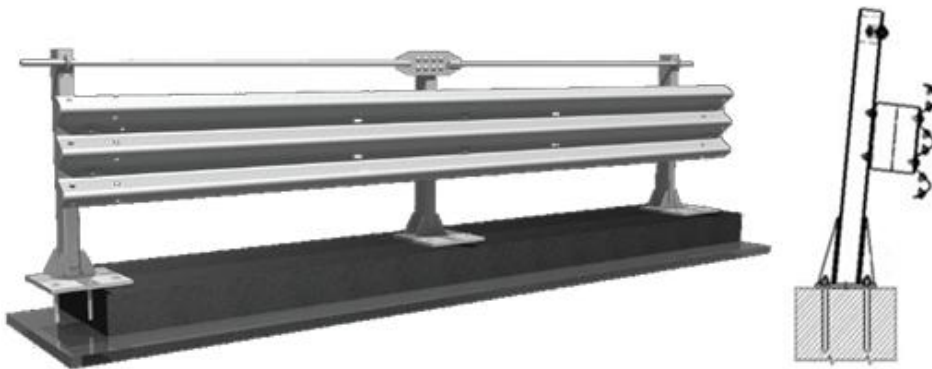
Figure 6.6. Installation technique of a bridge safety barrier.
