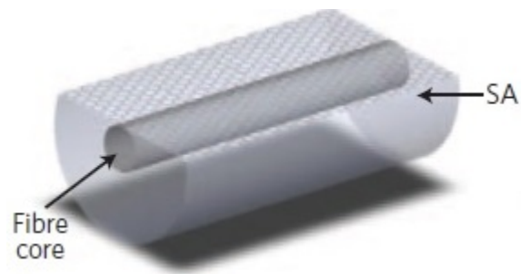
Figure 5.1: Deposition of a graphene SA on a D-shaped fibre. Adapted from Ref. [39]
