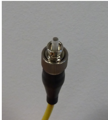
Figure 3.13: Graphene film transfer on fibre connector.
