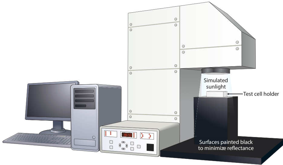
Figure 2.6: Typical set-up for the electrical characterization of a solar cell. Reproduced from [66].
