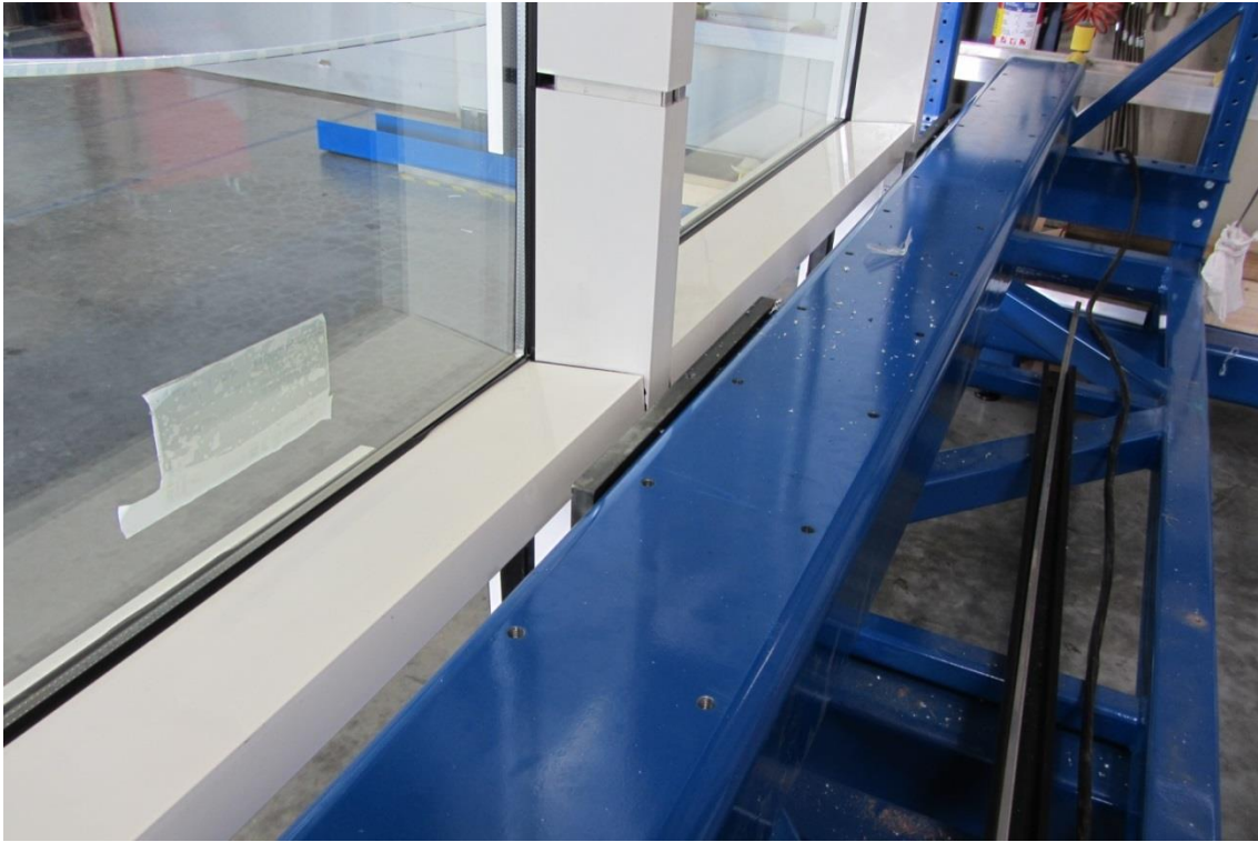
Figure 8-22: out-of-plane rotation of transoms (60 mm)
