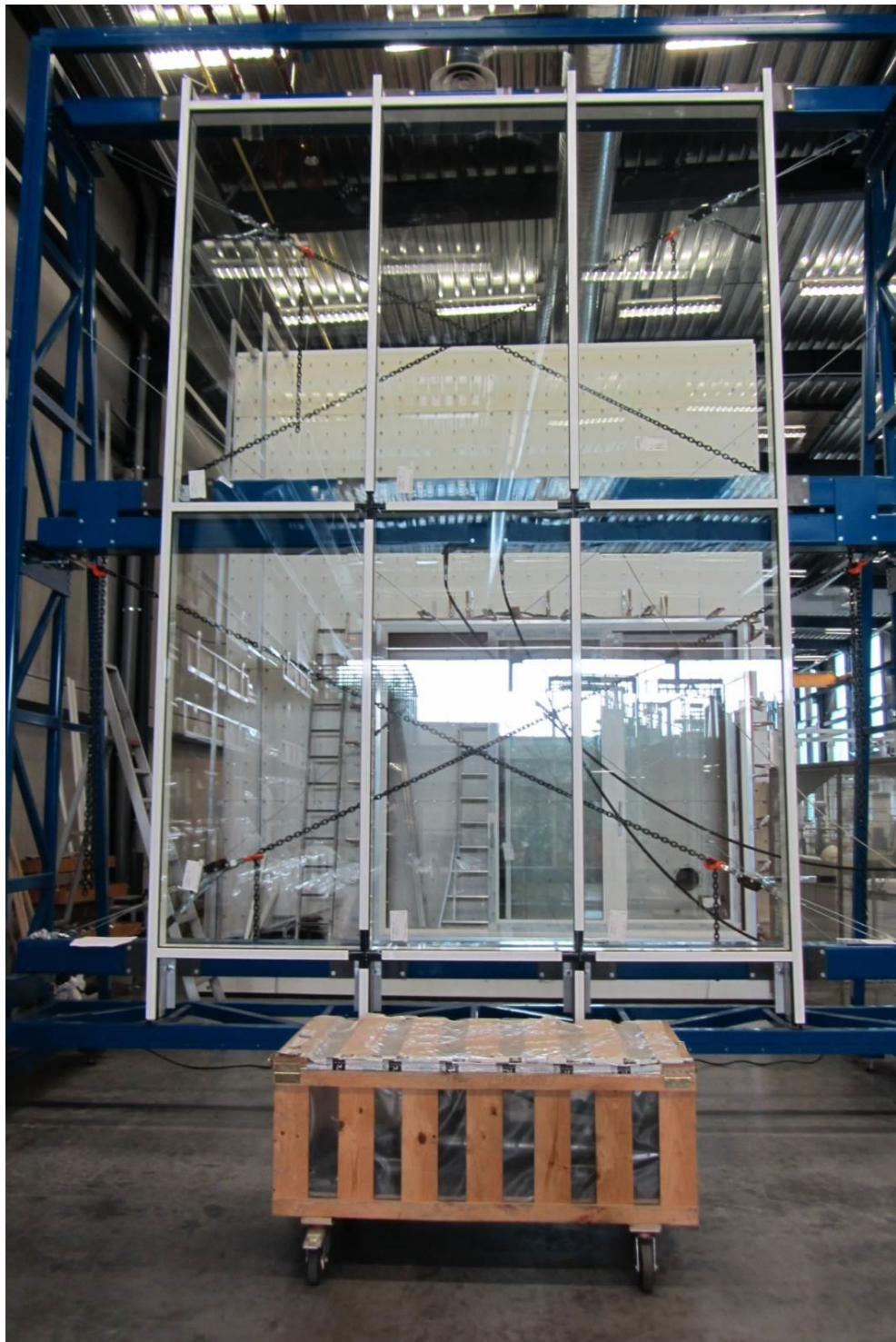
Figure 8-40: Picture of front view with the new double x reinforcement
