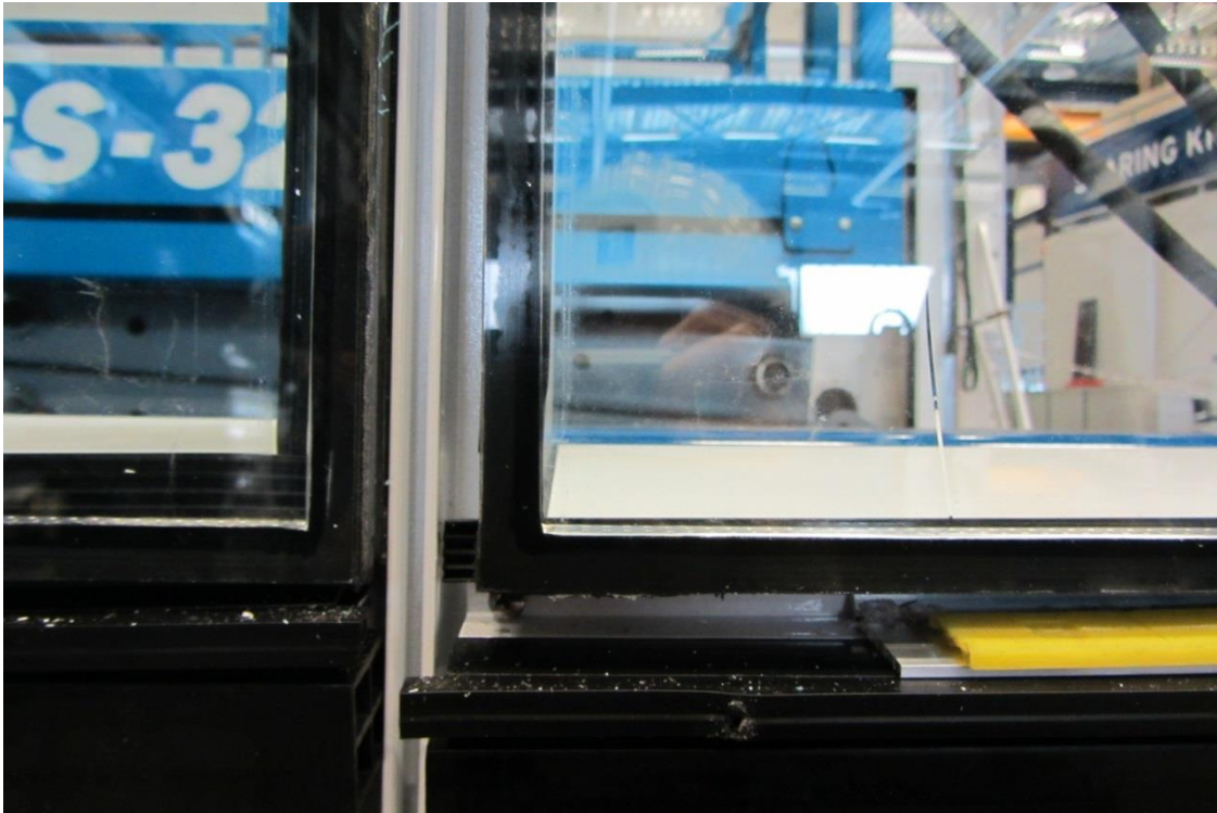
Figure 8-19: deformed frame and start of glass 3 breakage (15 mm)
