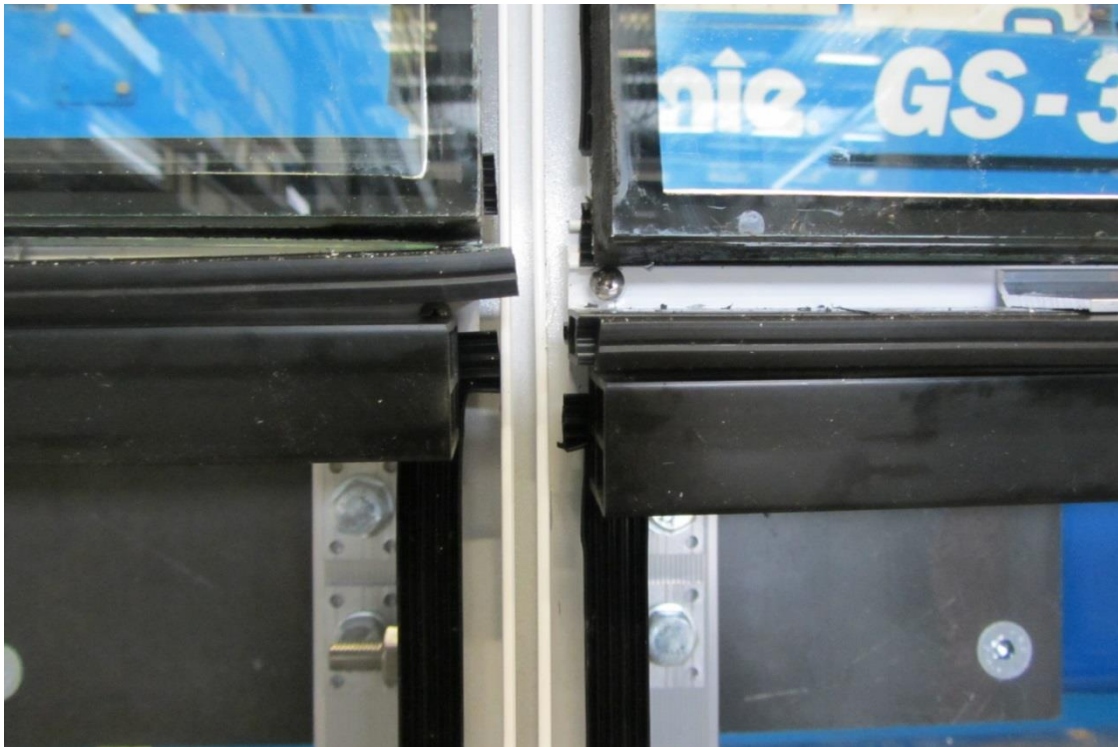
Figure 8-20: screw coming out under glass 3 (15 mm)
