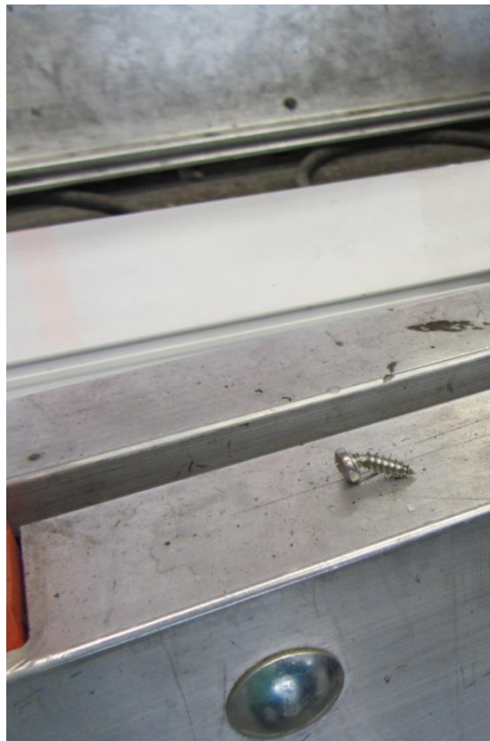
Figure 8-23: deformed screw (after dismounting)
