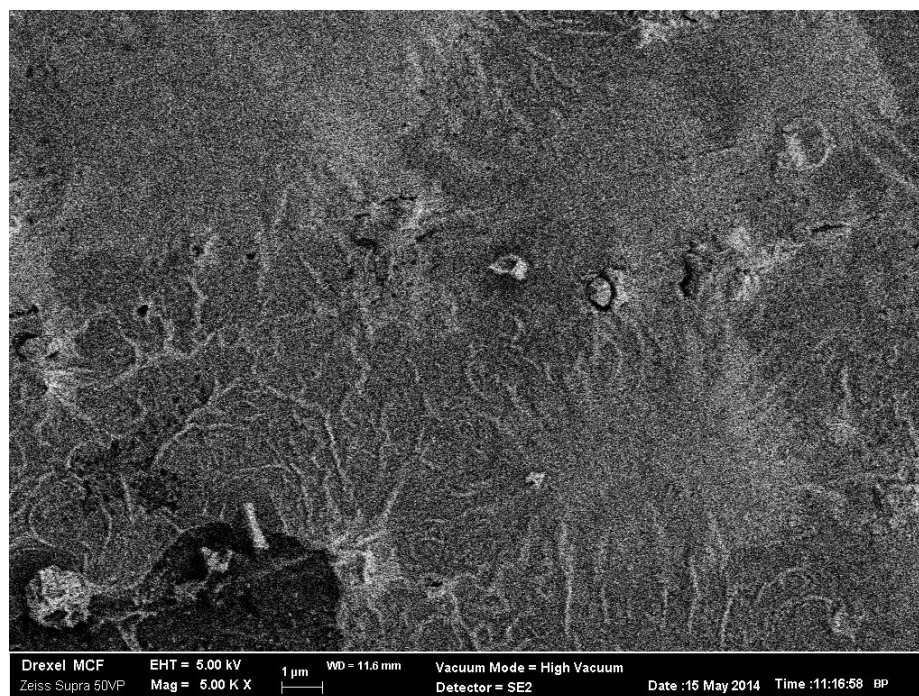
Figure 4.53 SEM micrograph of Cr/Au contact to p-GaAs ( N_A = 1.7 \times 10^{20} \text{ cm}^{-3} ), after 60 seconds of RTA at 500°C (5,000X)
