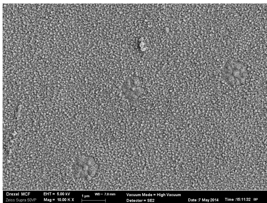
Figure 4.36 SEM micrograph of Au/Zn/Au contact to p-GaAs ( N_A = 4.0 \times 10^{16} \text{ cm}^{-3} ) after 60 seconds of RTA at 450°C
