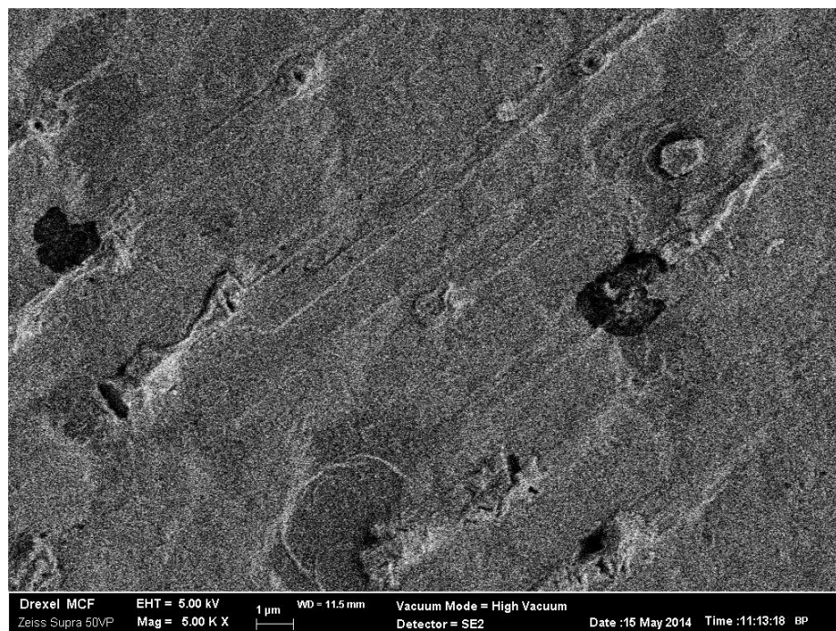
Figure 4.52 SEM micrograph of Cr/Au contact to p-GaAs ( N_A = 1.7 \times 10^{20} \text{ cm}^{-3} ), after 60 seconds of RTA at 450°C (5,000X)
