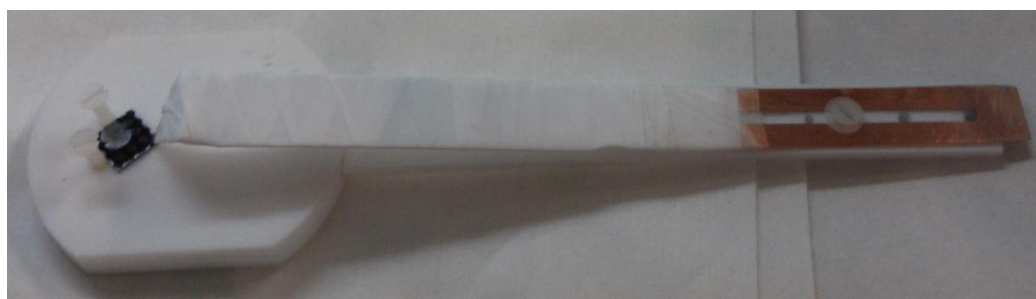
Figure 3.3 Sample holder used for GaAs IBSC wafers in electrolytic deposition experiment
