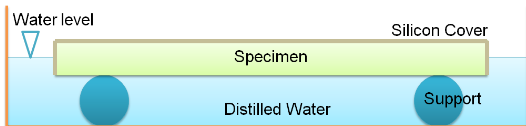
Figure 3.13 - Example of capillary absorption testing apparatus.
