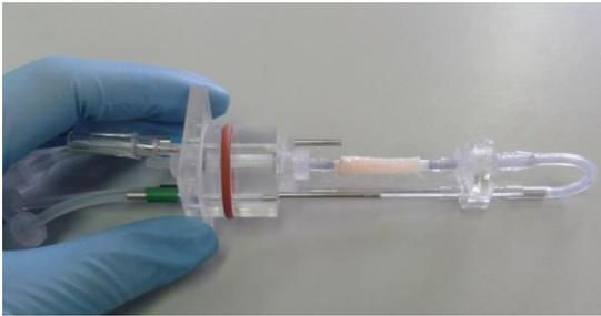
**Figure 8.** Porcine IMA sample fitted on the silicone sleeve and hosted between the two connectors on the vessel housing of the bioreactor.
