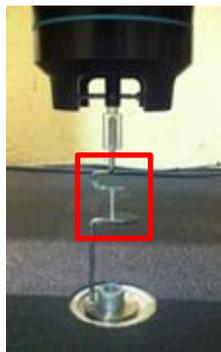
**Figure 9.** Ring tests setup. The biological sample is highlighted in the red rectangle.
