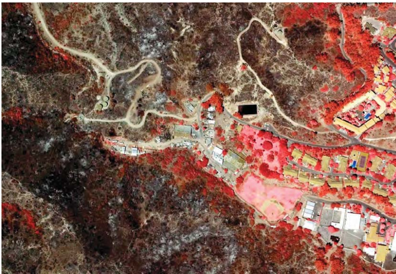
Figure 9.19: Near infrared photography for burned surface analysis.
