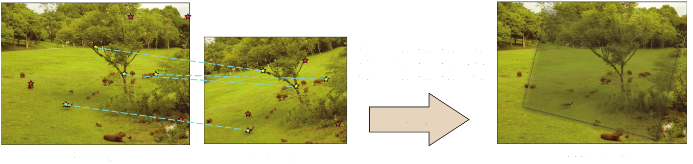
Figure 4.5: The near-duplicate registration process: we search for a geometrical transformation between I_n and I_m using SIFT matching (on the left) and we obtain the registered images (on the right).
