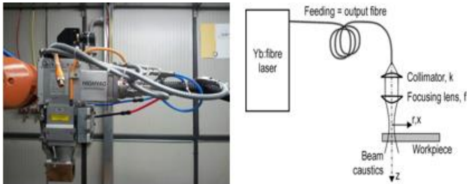
Figure 4-9 Bimo laser head, HIGHYAG laser technology, Laser delivery schematic
