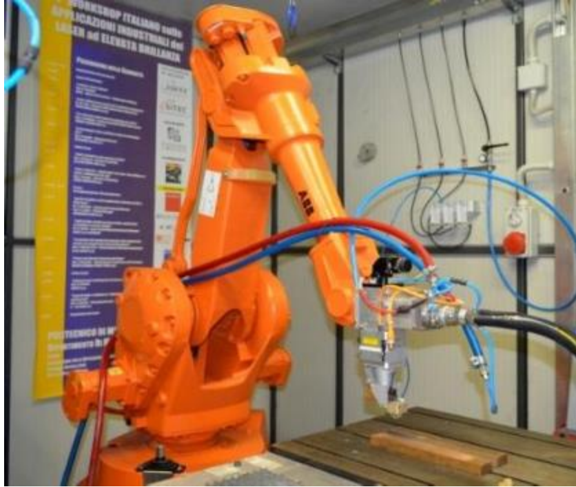
Figure 4-11 Laser annealing system set up
