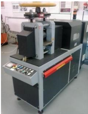
Figure 4-12 Cold rolling machine
