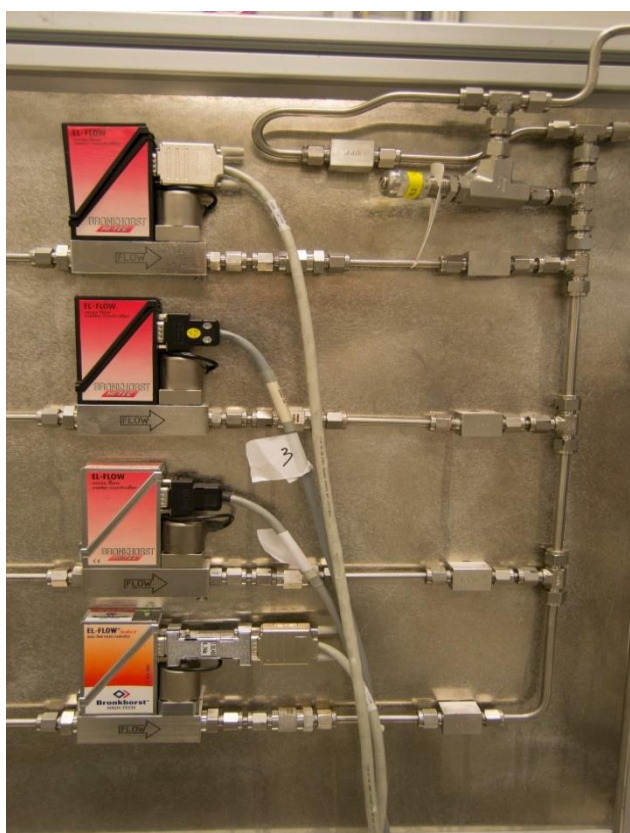
Figura 2.12: MFCs (Mass Flow Controllers)
