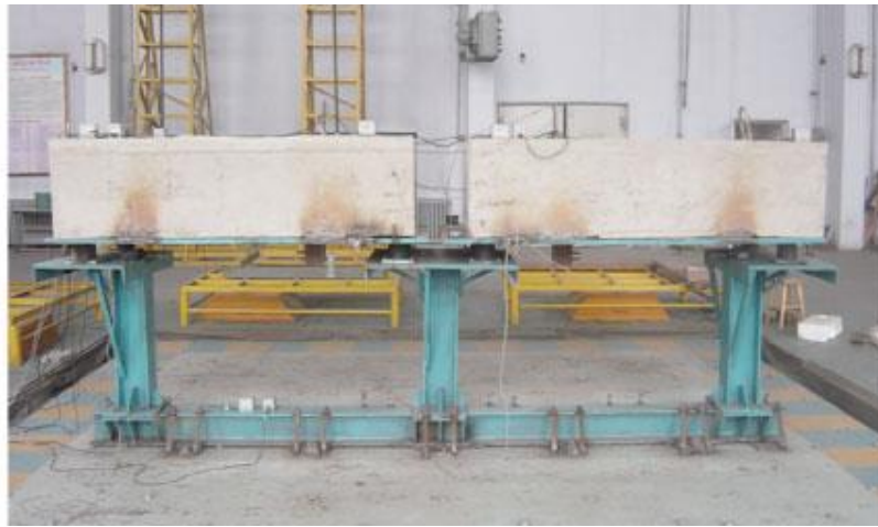
Fig. 2.23. Bridge model on the shaking table during the experiment at Harbin Institute of Technology.
