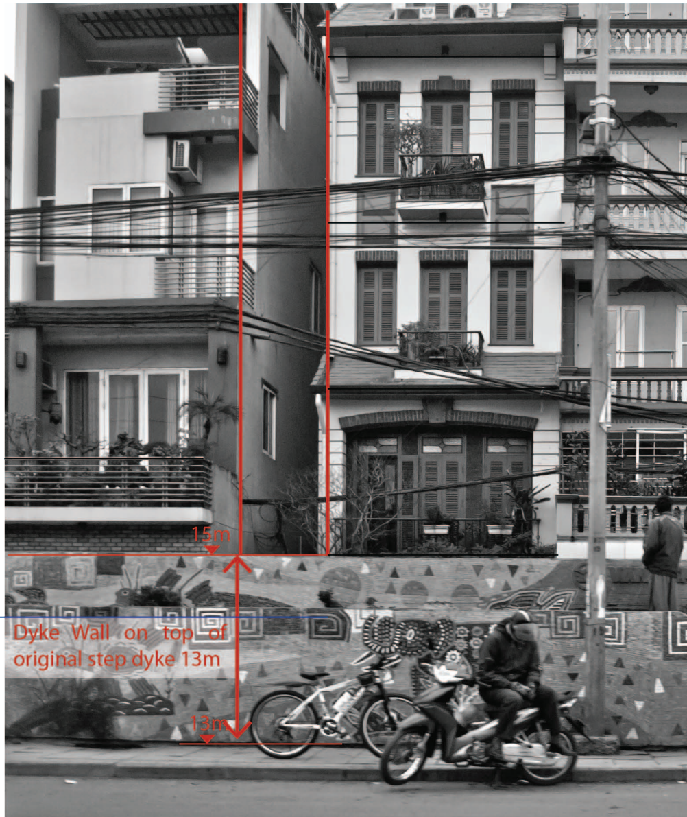
FIG. 4.5.3 Simulation of the eventual level of future extreme flood such as the one in 1971 in the higher located areas in RUA. Location Bach Dang ward, February 2014
