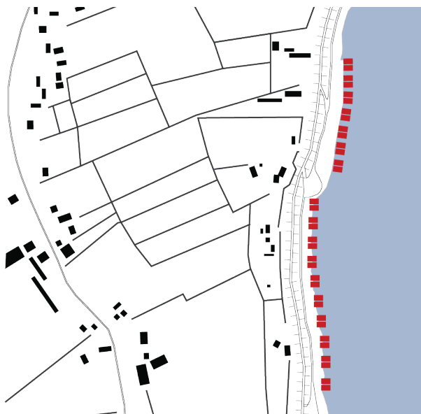
FIG. 4.4.2 Plan of the amphibious development in Maasbommel Source: Adopted from "Amphibious housing in the Netherlands" 68
