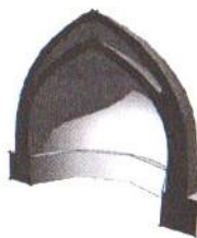
Figure 54: Continues double Shell dome
