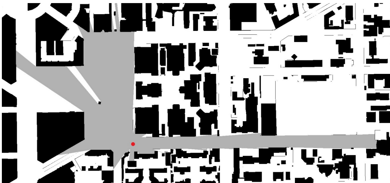
Figure 5.1 – Example of isovist from a point (Red), in grey the visible urban space; in white the occluding area; in black the obstacles.
