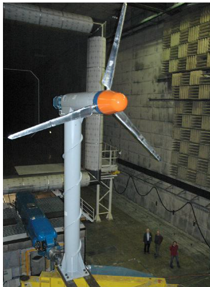
(A) MexNext wind tunnel model, test performed at LLF.
