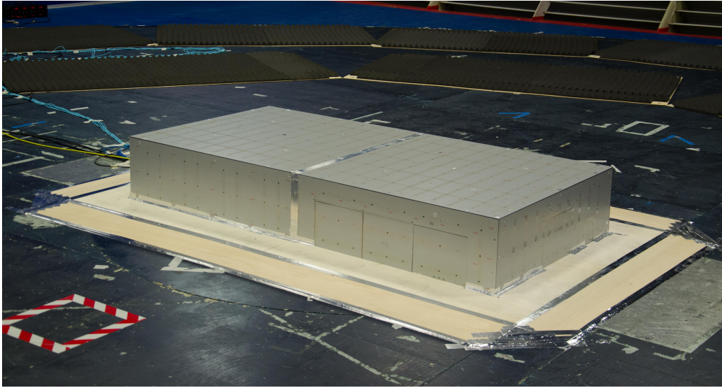
Figure 4.8: The hangar model used in the wind tunnel tests
