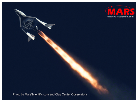
Figure 8.: SpaceShipTwo during the boost phase after separation from mother-aircraft [67].
