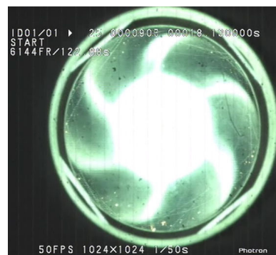
Figure 27.: Visualization of HTPB-based fuel combustion with swirling oxidizer (frontal strand section) with a frame rate of 50 fps.
