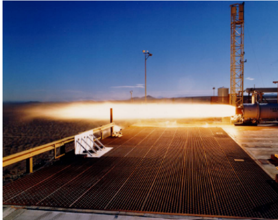
Figure 7.: AMROC H-500 motor firing test, propellant couple LOX/HTPB [55].
