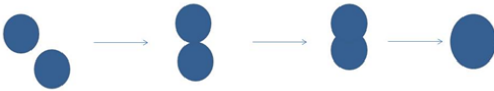
Figure 1-11 Steps of coalescence: approach, aggregation and finally coalescence.
